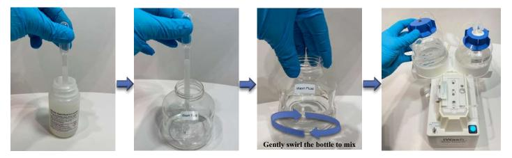
2.1.5 Pipette 2mL of silicone defoamer solution into the waste bottle and place in the right hand side of the white holder. Then gently screw on the waste bottle lid (lid with two pipes attached) until it is closed. Do not tighten the lid too hard. Closing the lid just when it stops turning is enough.
