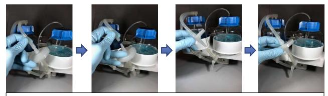
Changing the hydrophobic filter: Gently and slowly pull away the silicon pipes from the barbed ends of the blocked hydrophobic filter to remove it and then replace with a new hydrophobic filter by pushing the silicone pipes into the barbed ends of the new filter.
