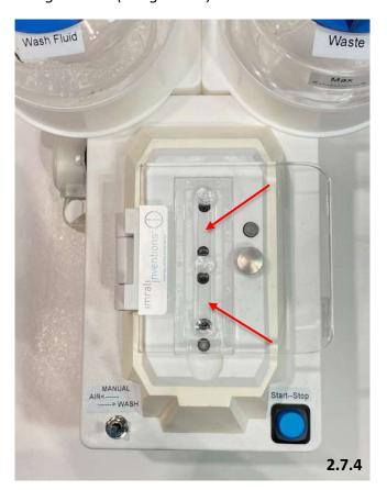
Top view of washer with a slide present in the slide loading chamber and the lid is in closed position. The arrows indicate the slide's chambers where the flow of wash fluid should be observed at the end of the priming step also during every slide washing cycle.
